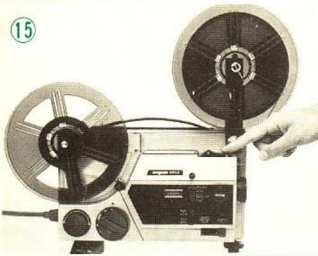
To reverse the direction of the film in order to see a portion of it that has been projected or for a special effect, turn the ROTARY POWER SWITCH to "R" and "L". To make the picture steady, where necessary, press down "R" of the LOOP FORMER (#15).
