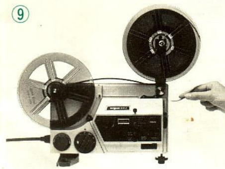
Turn the ROTARY POWER SWITCH to "F" and insert the trimmed end of the film into the FILM ENTRANCE (#9). As soon as the film has attached itself to the AUTOMATIC TAKE-UP REEL depress "F" of the LOOP FORMER (#11). Turn the ROTARY POWER SWITCH to "L" and you are ready for projection.
