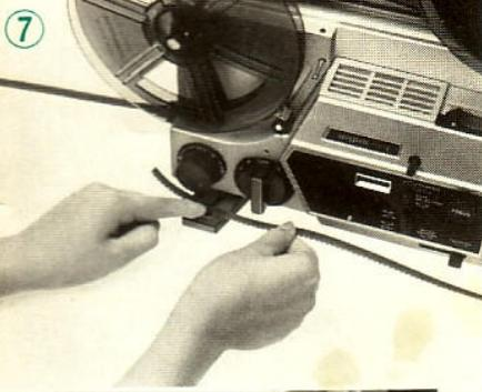
Place the end of the film under the FILM TRIMMER with one perforation over the small pin, and depress the spring blade (#7).
