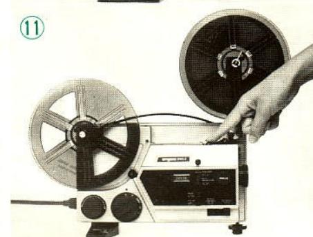
If the loop slips during projection, the picture will start jumping on the screen and a chattering noise will be noticed. Should this happen, press down a few times "F" of the LOOP FORMER during forward projection, and "R" during reverse projection until the picture becomes steady once again. Make sure to press down "F" as soon as the film has attached itself to the AUTOMATIC TAKE UP REEL (#11).
