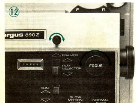
The projector is equipped with an f/1.5 20-32mm zoom lens. To zoom the lens, slide the lens barrel back and forth until the picture fills the screen to the desired image size. To focus the picture, rotate the FOCUSING KNOB until the projected image is sharp and clear (#12). If the picture is high or low on the screen during projection, rotate the FRAMER until the picture is properly centered on the screen (#12).
