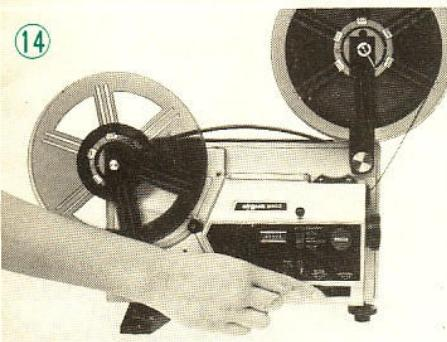
For slow motion projection, move the SLOW MOTION LEVER from "NORMAL" to "SLOW MOTION". The speed may be reduced down to 4 frames per second by adjusting the VARIABLE SPEED CONTROL DIAL. Slow motion pictures may be enjoyed both during forward and reverse projection. After slow projection, be sure to move the SLOW MOTION LEVER back to "NORMAL" (#14). \*(890Z only)
