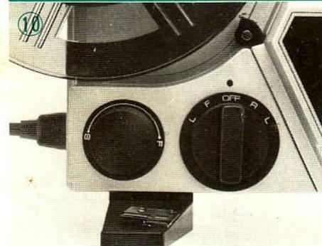
For forward projection, turn the ROTARY POWER SWITCH to "F" and then to "L". For reverse projection, turn the ROTARY POWER SWITCH to "R" and then to "L". To stop the motor and lamp, turn it to "OFF" (#10). Turn the VARIABLE SPEED CONTROL DIAL to "F" to increase the speed or to "S" to reduce it. Normally the speed control should be set halfway between "F" and "S" (#10).
