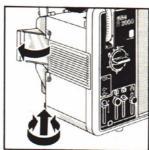
Remove the lamp cover and rear panel. Remove the projection lamp from its holder. Remove the worn drive belt and place the new belt in the pulley groove corresponding to your line (mains) fre-
